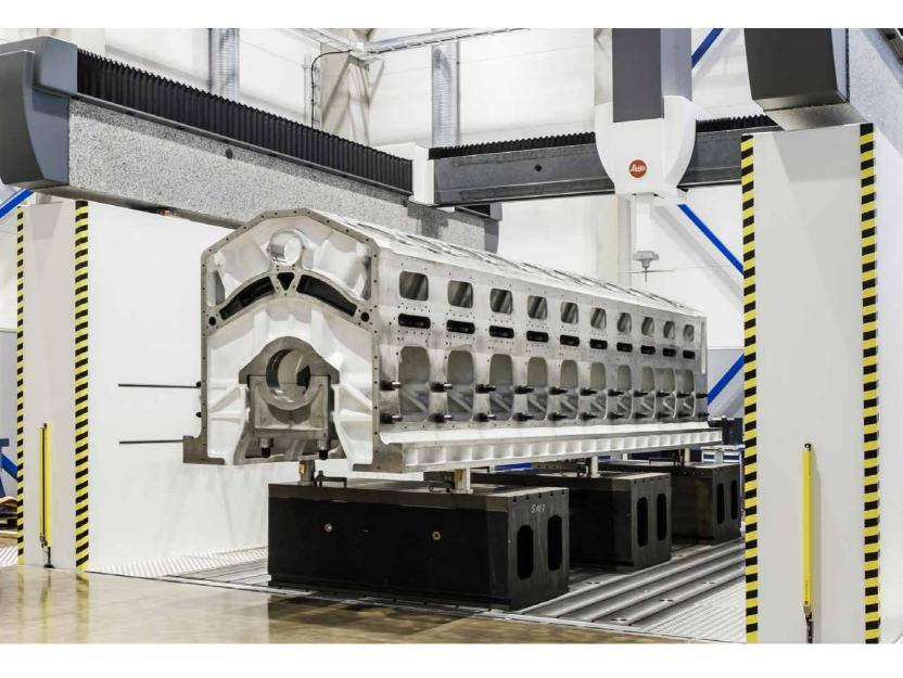
We ensure the geometry and dimensional tolerances of our components within a precision of thousandths of a millimetre. We have a comprehensive range of conventional and geometrical measurement devices in house.
